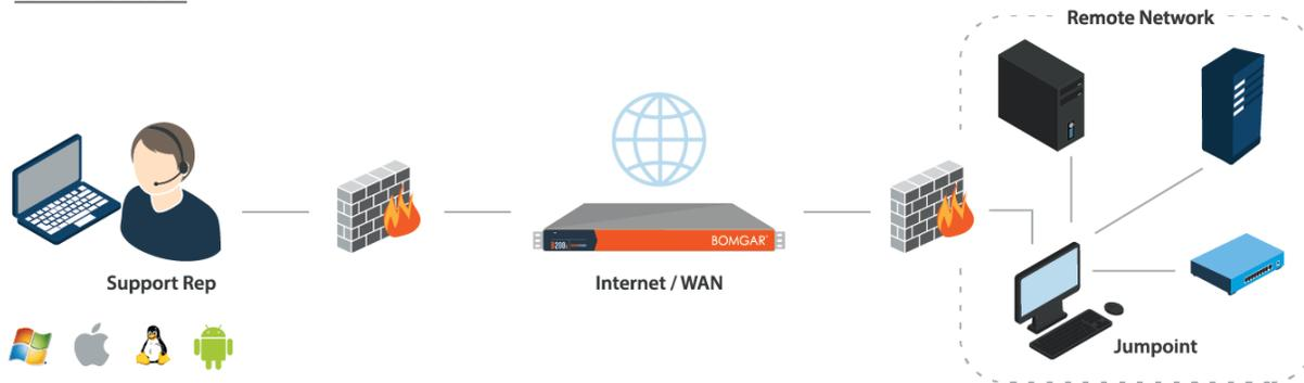
A Jumpoint acts as a conduit for access to computers on a known remote network. A single Jumpoint installed on a computer within a LAN is used to access multiple systems, eliminating the need to pre-install software on every computer you might need to access.
