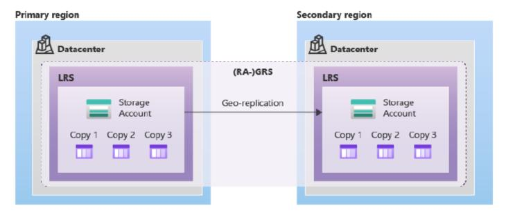
Data in the secondary region is not directly accessible to users or applications (read access), unless a failover occurs. The failover process updates the DNS entry provided by Azure Storage so that the secondary endpoint becomes the new primary endpoint for your storage account. During the failover process, your data is inaccessible. After the failover is complete, you can read and write data to the new primary region.
