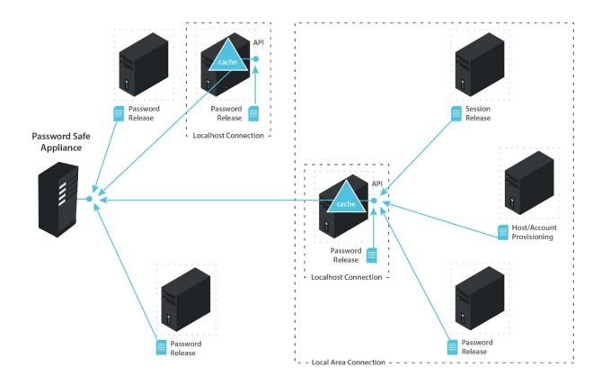
Each Cache can store credentials that may be released in an emergency. A synchronized storage option for the Worker node is planned for a future release of Password Safe.
