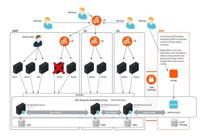
UVM appliances connect independently to the database and contain the web interfaces and processes that allow end users to interoperate with the solution. Typical use case scenarios are:
