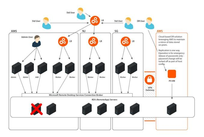
If a RemoteApp (Remote Desktop Server) were to fail, Microsoft RD Connection Brokers may be used to failover a user session to an alternate host. Another method is to add load balancers between the Session Proxy (on the Worker node), and the RemoteApp Servers.
