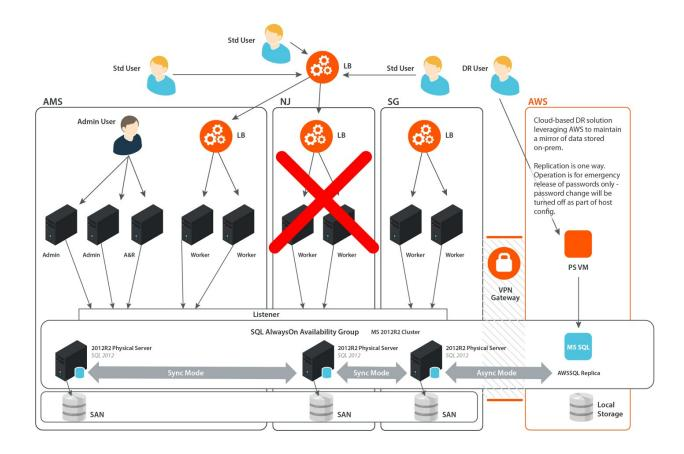
In the event that a secondary site were to go offline, users would be automatically re-directed by the load balancers to either one of the alternate sites in operation.
