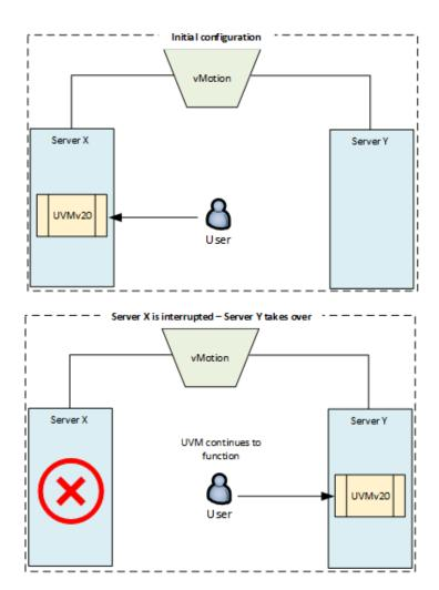
VMware vMotion can be used to keep the UVM virtual appliance continuously available even if the physical server running the virtual image goes offline for any reason. As seen above, the UVM virtual image is deployed to ESX Server X. This server is continuously mirrored to Server Y such that if a hardware failure were to occur, the virtual image continues to be available as if nothing happened.
