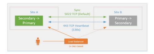
If it is desired that roles be reverted, wait for replication to complete then the following manual steps are performed:
