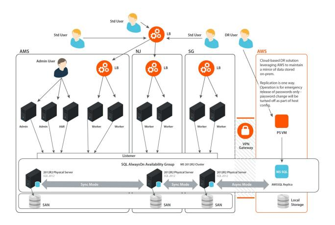
In this example, UVM appliances in each of the three primary datacenters Amsterdam, New Jersey, and Singapore, are connected to a MS SQL AlwaysOn Availability Group. Note that each appliance can initially assume any mix of roles and may be reconfigured at any time after deploying into production.
