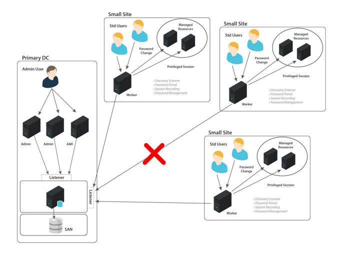
In the current architecture, any separation from the central database will prevent users from logging on to the Worker node.
